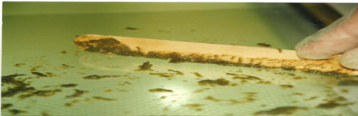
Thick fouling deposit on the membrane surface
